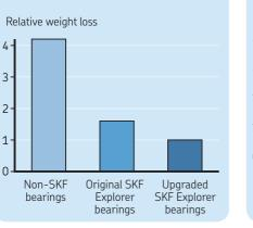
Relative wear for different bearing steel
