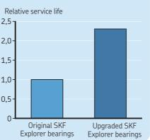
Service life under poor lubrication
