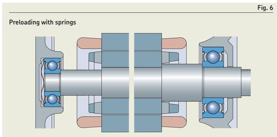
For small electric motors, values of between 0,005 and 0,01 are used for the factor k. If preload is used primarily to protect the bearing from the damage caused by external vibrations when stationary, then greater preload is required and  $k = 0,02$  should be used.
