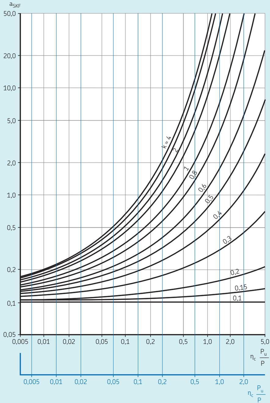
Factor  $a_{SKF}$  for thrust ball bearings
