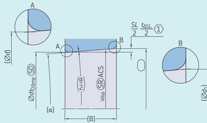
$$\textcircled{1} = \begin{cases} SL \text{ is a calculated nominal size from } d \text{ and } d_1, \text{ i.e. } SL = (d_1 - d) = 2B \tan(\alpha/2); \\ \Delta SL \text{ is a calculated characteristic, i.e. } \Delta SL = \Delta d_{1mp} - \Delta d_{mp} \end{cases}$$
