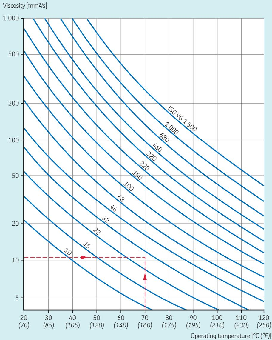
Estimation of the rated viscosity  $v_1$
