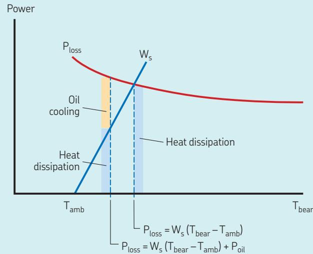
If you do not have values for  $T_{out}$  or  $T_{in}$ , you may assume a temperature difference of 5 to 10 °C (10 to 20 °F).
