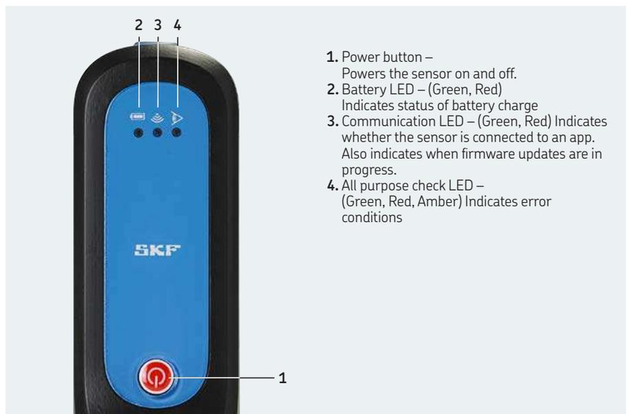
1. Power button – Powers the sensor on and off.
