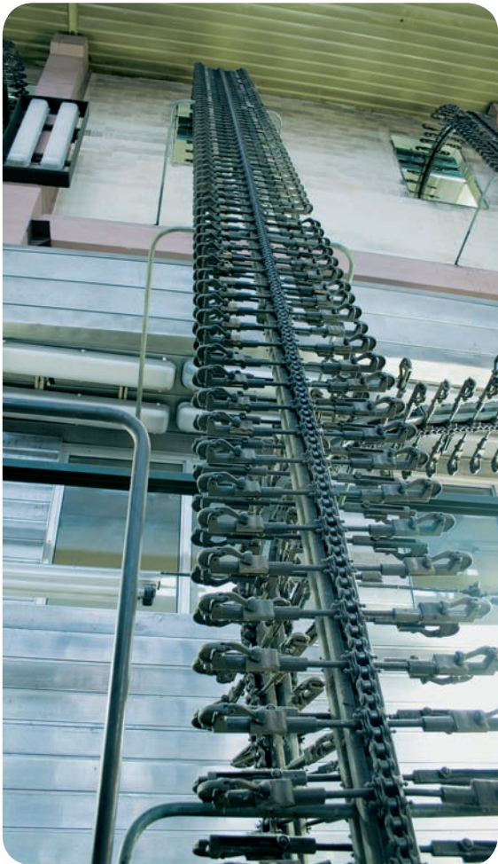
Hollow pin chain used on a newspaper conveyor
