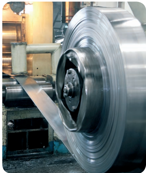
Continuous rolling machine to achieve uniform thickness of plate material
